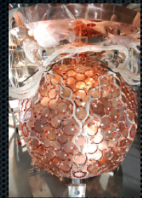
XMASS at Kamioka: 835 kg LXe (100 kg fiducial), single-phase, 642 PMTs unexpected background found detector refurbished new run this fall -> 2013
